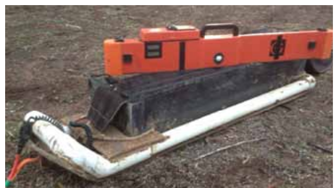
Picture 1: An EM38-MK2 mounted on a sled for survey work.
