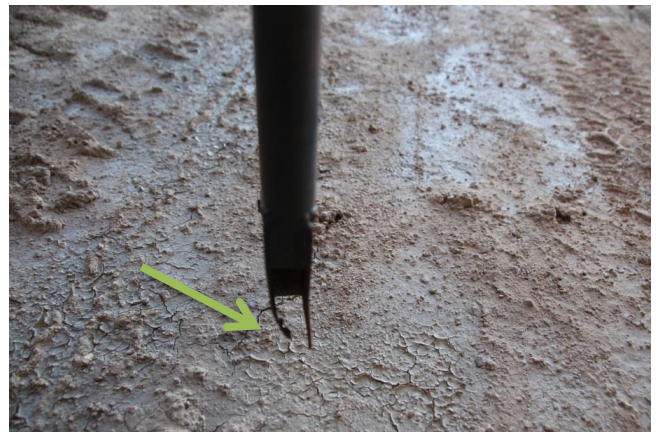
Figure 5: Wear and deformation (arrow) on this boot may inhibit seed flow.
