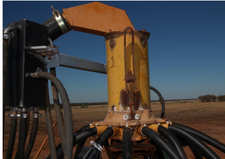
Figure 7: An over centre catch was installed on this distributor to allow blockages to be cleared quickly.
