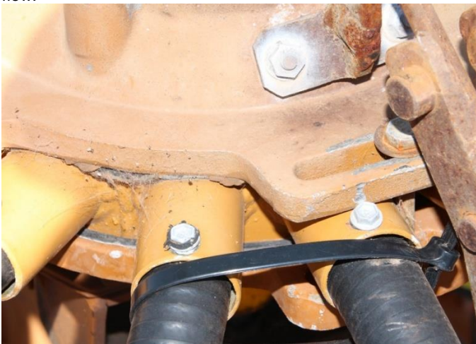
Figure 3: Tech screw used to fix hoses may impede seed flow.
