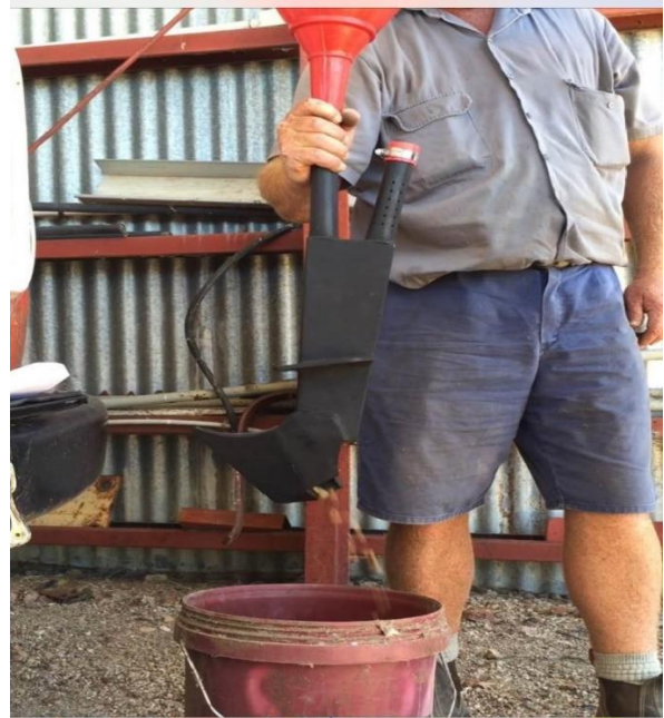
Figure 4: Testing a tyne/boot assembly with faba bean seed.
