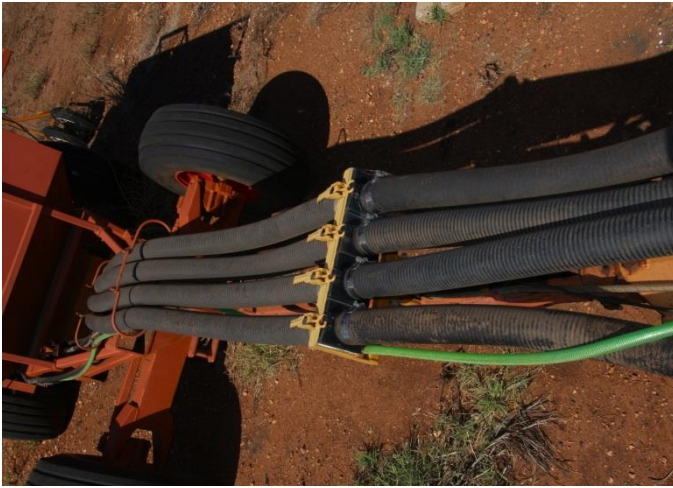
Figure 2: On this machine four hoses run from the cart eliminating the need for splitters.
