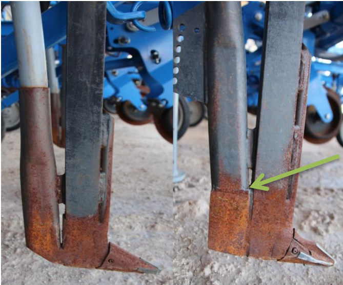
Figure 6: One piece construction (left) are more suited to faba bean. Welds on tynes (right) may protrude on the inside and restrict flow.
